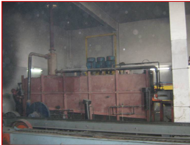
Figure2.1: Energy efficient gas fired reheating furnace
